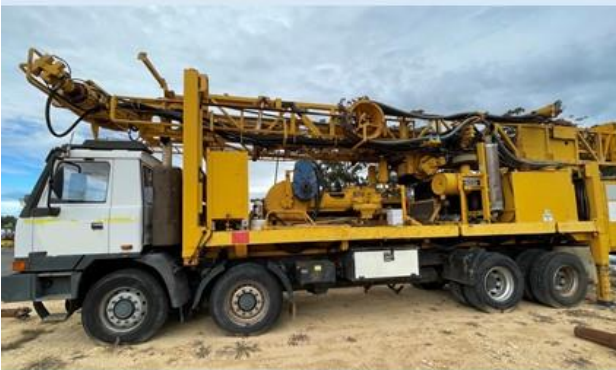
Pictured: UDR1000 multipurpose rig, dump mast equipped set up for water-boring, on Tatra 8x8
